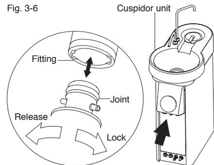
Note: Clean the joint if it is difficult to connect the vacuum hose, or the saliva ejector hose, back to the cuspidor unit.
