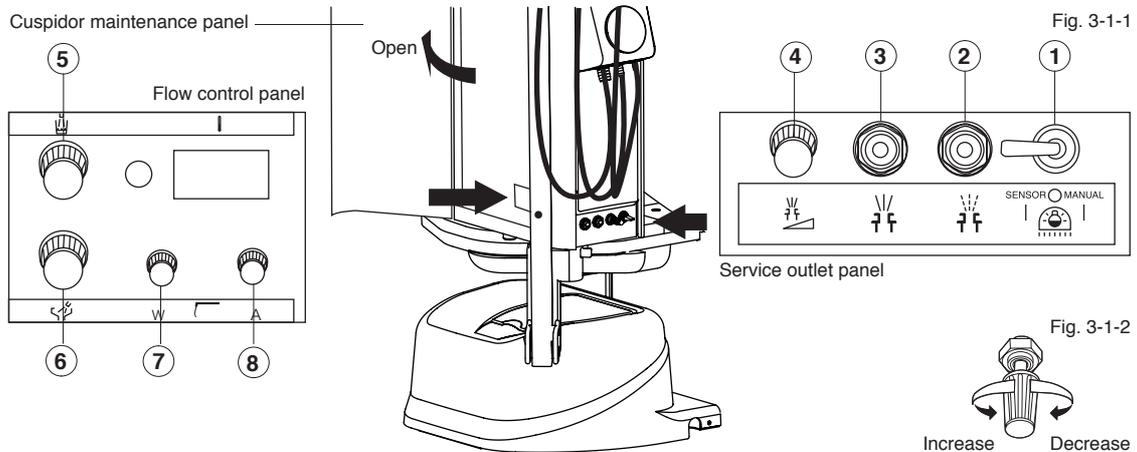
① Dental light on/off and sensor mode switch
