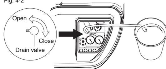
Note: Failure to drain off the water from the air filter bowl could affect the performance the handpieces.
