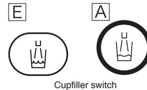
Note: Cupfilling as well as cuspidor bowl flushing are cancelled when the cupfiller switch is pressed while the functions are activated.
