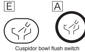
Note: Cuspidor bowl flushing is terminated immediately when the cuspidor bowl flush switch is pressed in either mode.
