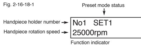
Note: When the micro motor is returned to its holder the selected speed setting will be stored until re-selected or until the unit is switched off. Alternatively the selected micro motor preset speed can be stored as a default setting.
