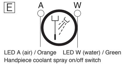
For micro motors, the mode can be selected from 2 different modes, i.e. 2-mode (Fig. 2-16-14-1) and 4-mode (Fig. 2-16-14-2), and handpiece coolant spray setting is sequentially switched to 4 different settings, i.e. spray on, water only, air only and spray off, each time the handpiece coolant spray on/off switch is pressed if 4-mode is selected.
