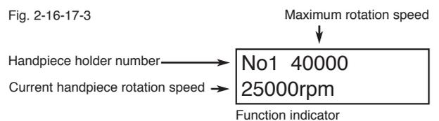
Note: the maximum rotation speed and the actual speed of the micro motor will be displayed in the function indicator. (Fig. 2-16-17-3)
