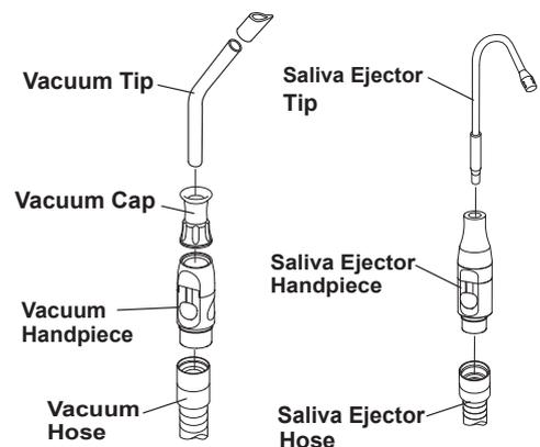
Fig.5-3 Vacuum Handpiece and Saliva Ejector Handpiece
