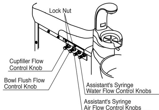
Fig.3-20 Flow Control Knobs in Cuspidor Unit Body
